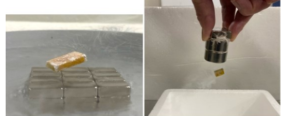
Fig.1 Magnetic flux pinning phenomenon in pseudo-bulk superconductors.
