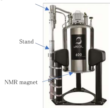
Fig.2 Photo of the Cryogen Reclamation System attached to an NMR magnet.
