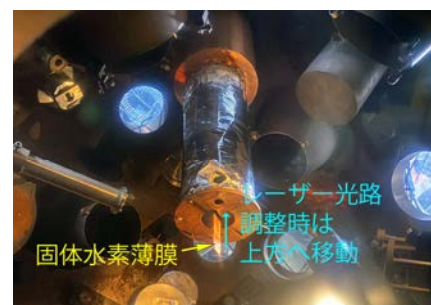
Fig.3 Thin film solid D 2 target.
