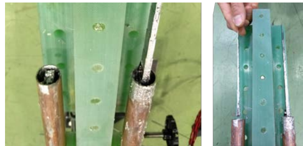
Fig. 2. Burned REBCO tape. The root of the left side was burnt to torn off.
