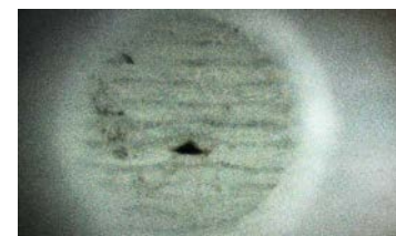
Fig.3 Dielectric breakdown path at LNT.
