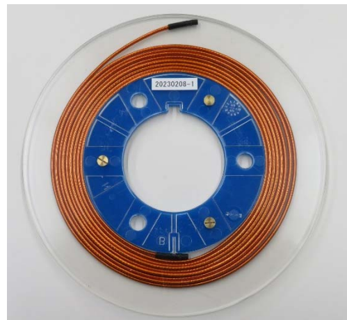
Fig. 2 5 m-long mock-up cable made with copper tapes.
