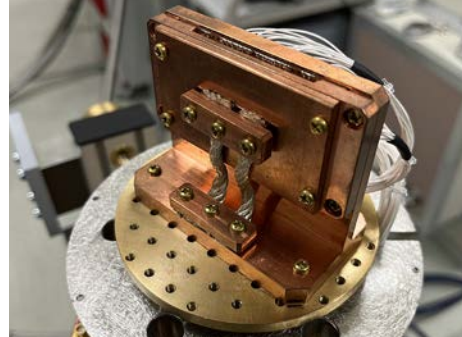
Fig. 1 Package holder mounted on the 0.3-K stage of a 3 He cryocooler (the package is equipped with 48 cables).
