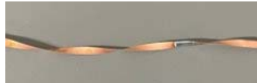
Fig. 2. Photograph of a 4mm-width REBCO coated conductor after I_c vs torsion angle measurement.
