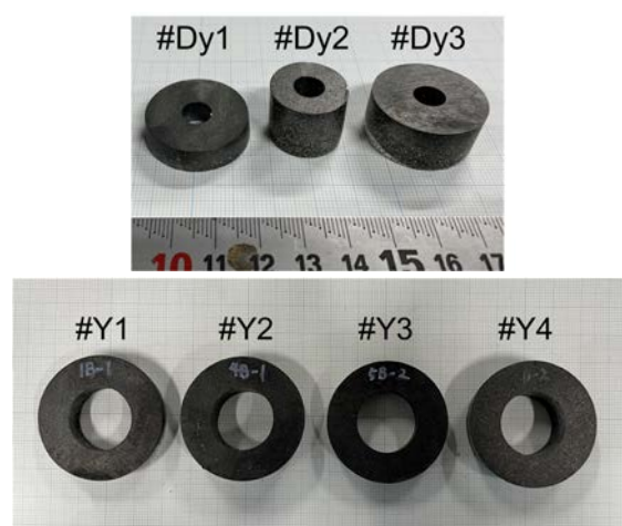
Fig. 1. Appearance of SDMG-processed DyBCO and YBCO melt-textured ring-bulks fabricated using ring-shaped dies with outer and inner diameters of 25 mm and 10 mm (#Dy2), 35 mm and 10 mm (#Dy1, 3), and 50 mm and 25 mm (#Y1–4).
