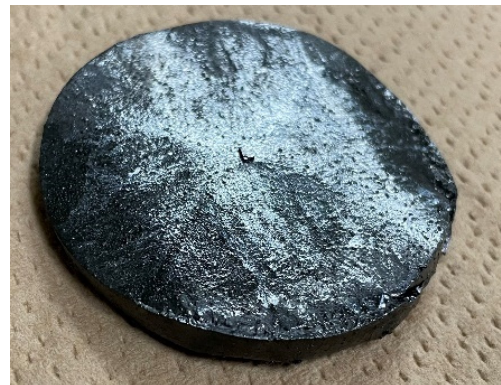
Fig. 1. (Y, Er)BCO bulk fabricated by RE composition gradient method
