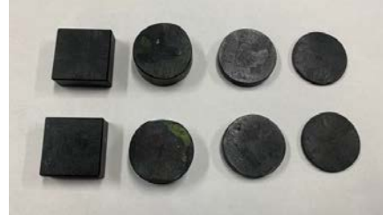
Fig.1 Photograph of superconducting bulk material for magnetic shielding (Thickness from left to right: 10mm 10mm 5mm 2mm)
