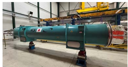
Fig. 2. MBXF cold mass prototype assembled into the cryostat.
