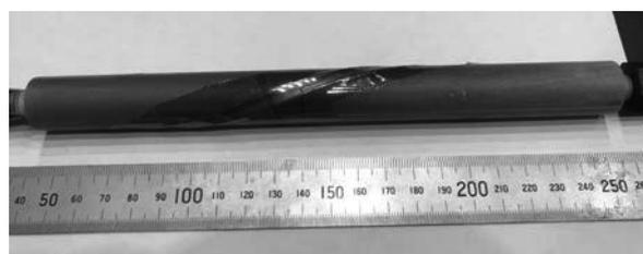
Fig.4 Spirally wound multi-filament coated conductor
