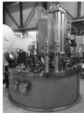
Fig.2 Liquid Nitrogen circulation system
