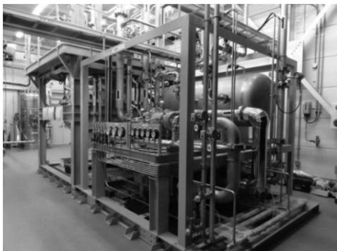
Photo.1 Turbo-Brayton refrigerator for test
