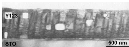
Fig. 3 Cross-sectional TEM image of an oxygen annealed Y123 film after annealing at 700°C for 1 h under  $P_{O_2} = 10$  Pa.
