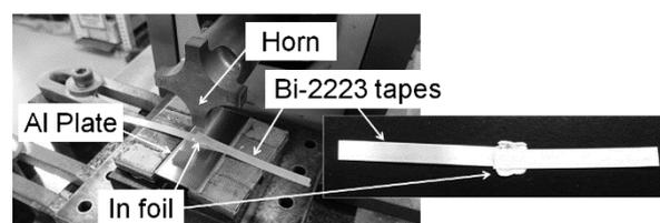
Fig. 1 Ultrasonic welding machine and its joint sample.
