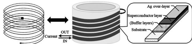
Fig. 1 Structure and schematic diagram of nonintersecting type non-inductive winding type based REBCO coil.
