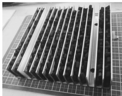
Fig.1 Test specimen of the activated carbon
