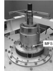
Fig. 1 Basic structure of Magnetic fluid seal. Fig.2 Magnetic fluid seal on FESS
