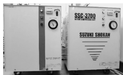
Fig. 1. Photographs of two types of the compressors. The left side shows C300G (rotary) and the right side shows SSC3700 (scroll).
