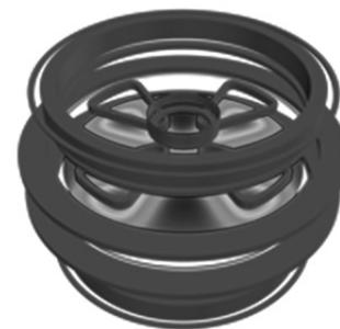
Fig. 3. Schematic drawing of HTS coil system for K80 Skeleton Cyclotron
