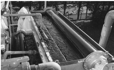
Fig. 1 Real Scale Magnetic Separator (200 m<sup>3</sup>/d)
