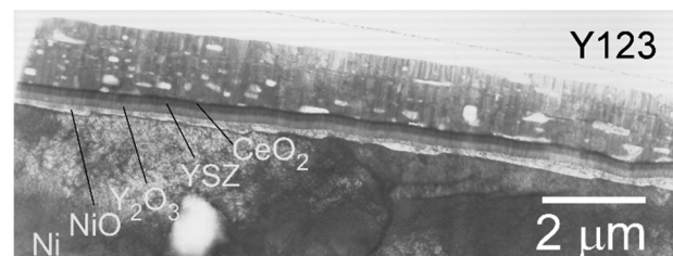
Fig. 3 Cross-sectional TEM image of Y123 film ( \sim 1.5 \mu\text{m} ) prepared by the triple-sintering method.
