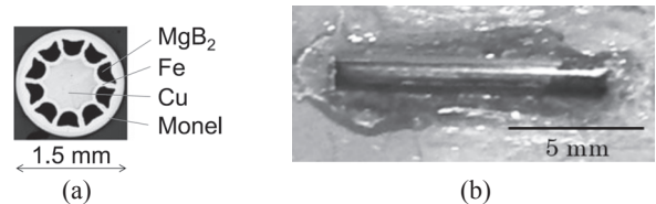
Fig. 1. Photographs of the sample: (a) the cross section [1], and (b) a 10-mm-long piece for the measurement.
