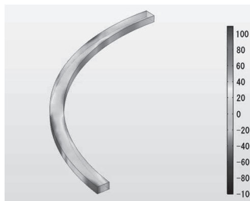
Fig.3 Hoop stress distribution of a coil when the number of additional bolts was one.
