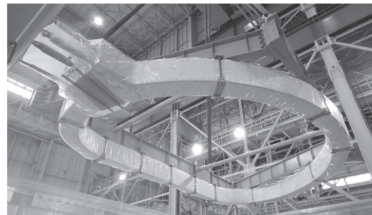
Fig.3 2 nd ITER TF coil WP after WP insulation.
