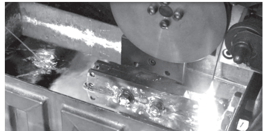
Fig. 3 Reel to reel RHQ treatment in an open air.
