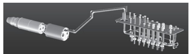
Figure 3. Two LHe Vessels of the SC magnet cryostat and Current leads, control valves, and instrument wires in the service cryostat
