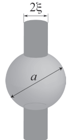
Fig. 3 Schematic showing the interaction between a flux line and a relatively large sphere pin.
