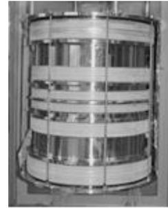
Fig.1 Photograph of a conduction-cooled REBCO coil
