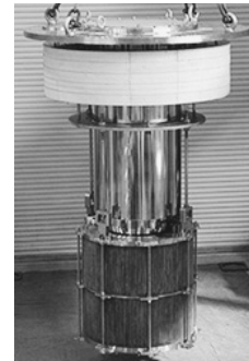
Fig. 2 13T magnet with 700 mm bore diameter
