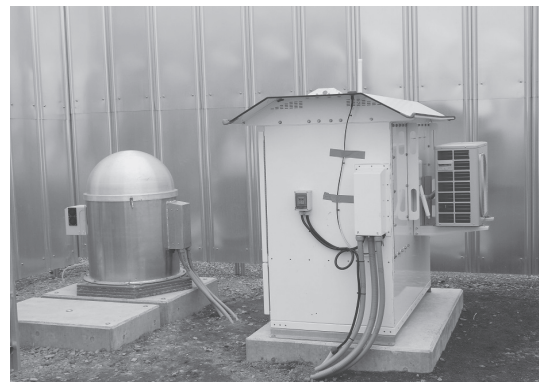
Fig.2 Field type Superconducting Gravimeter
