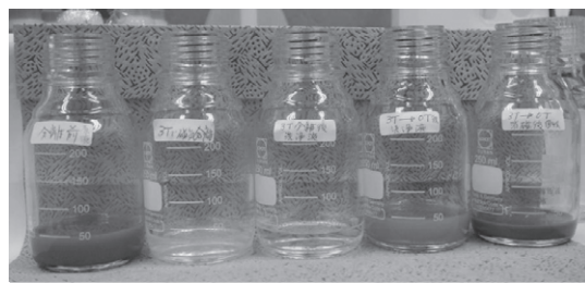
Fig. 3 Result of solutions in each process: (a) undiluted solution, (b) recovered solution under a magnetic field of 3 T, (c) recovered solution after flushing under a magnetic field of 3 T, (d) recovered solution after flushing in a zero magnetic field and (e) recovered solution after demagnetization of the filter and flushing.
