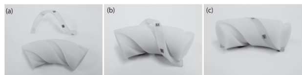
Fig.4 Photo images of the 3D printer models used for the feasibility study of segmented fabrication of the helical coil.
