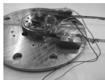
Fig.1 Photograph of fabricated small-sized GdBCO double pancake coil (turn number: 30, inner diameter: 50 mm, outer diameter: 65 mm, height: 10 mm)
