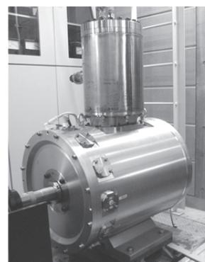
Fig. 2 Photograph of a 20 kW class HTS-ISM considered for analysis.
