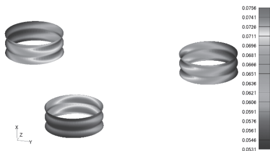
Fig.3 Calculated eddy current (3D, eccentricity: 0mm).
