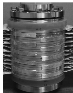
Fig.1 Photograph of small-bore 10 T superconducting coil
