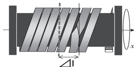
Fig. 2 two-strand parallel conductor wound into a 1-layer solenoidal coil
