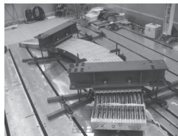
Fig.3 Test for CP welding of rRP curved mockup.
