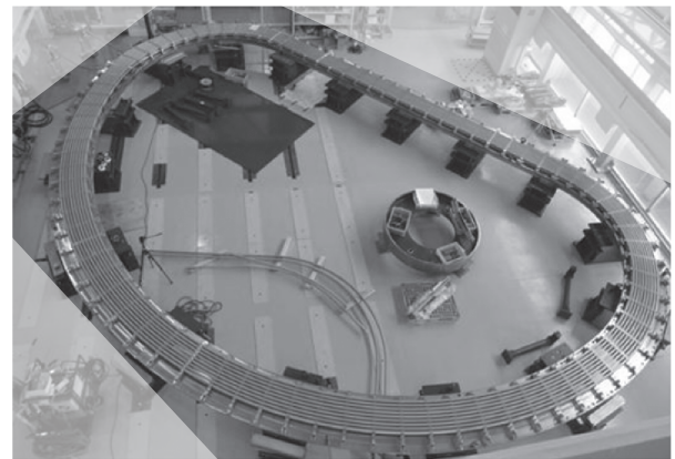
Fig.1. Fabricated side DP winding for DP7 of TF01.
