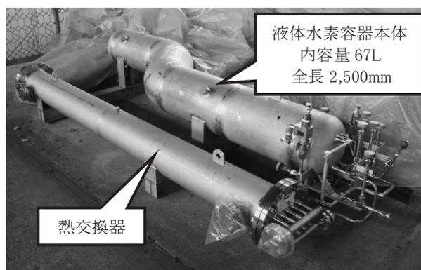
Fig.1 Overview of liquid hydrogen cryogenic tank
