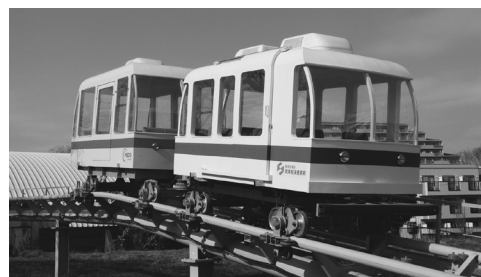
Fig.4 “Eco-Ride” New concept of guided public commuting system with roller coaster technology
