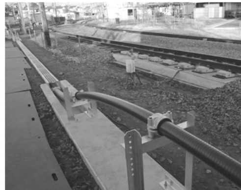
Fig.2 Photograph of 30-m superconducting cables in a railway test track
