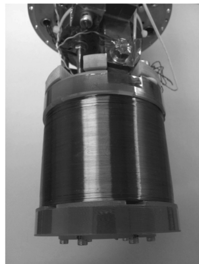
Fig. 1 Photograph of Bi-2223 superconducting coil on the test probe.
