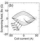
Fig. 2 Effect of *n*-value on the screening field (simulated results). (a) Non-scribing. (b) With scribing.
