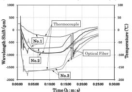
Fig.2 Result, Time Variations of Wavelength Shift and Temperature (WDM Type)
