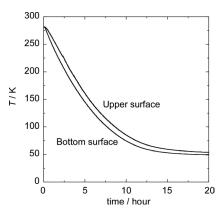
Fig.3. Cooling test of 5 layer bulk superconductor annuli
