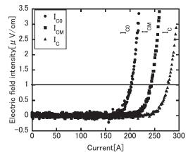
Fig. 2 V-I characteristics for critical current
