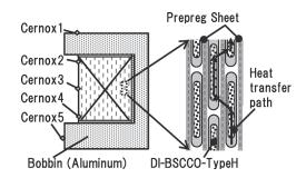
Fig.1 Structure of coil windings and setup of temperature sensor
