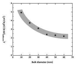
**Fig. 2.** Bulk diameter dependence of averaged current density at 20 K estimated from the trapped field values.
