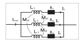
Fig.1 Equivalent circuit of a 3-strand parallel conductor
