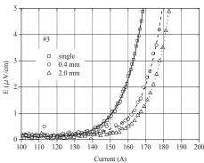
Fig.2 E-I curves for single and five tapes conductor with different gaps
