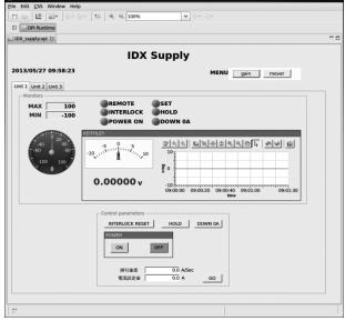
Fig.3 Control screen for the IDX magnet power supply.
