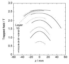
Fig.1. Trapped field of multi layer bulk superconductor annuli
