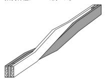
Fig.1 A transposed two-strand parallel conductor
