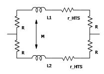
Fig.3 Equivalent circuit of a 2-strand parallel conductor
