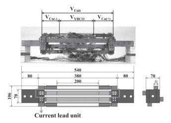
Fig. 1 Assembled superconducting current lead.
