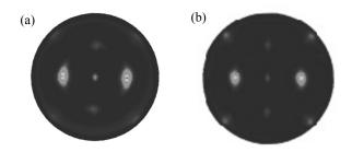
Fig.2 Pole figure mapping of the (017) reflection for the magnetically aligned Er124 ceramics in MRFs ( $\mu_0 H_a = 3$  T,  $\Omega = 20$  rpm) with (a) the unidirectional rotation type and (b) oscillation type.
