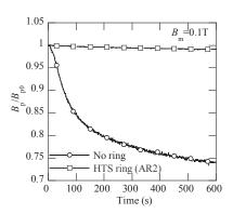
Fig. 3 Time evolutions of  $B_p/B_{p0}$  of bulk with and without shielding ring.
