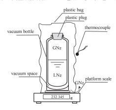
Fig. 1 Illustration of measuring device of liquid nitrogen evaporation amount in a drinking cold vacuum bottle
