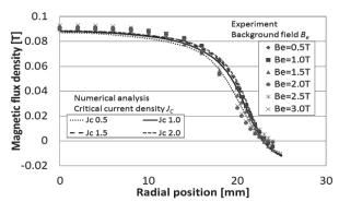
Fig.1 Comparison of the analysis and experimental results of magnetic flux density distribution
