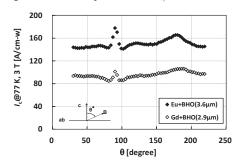
Fig.2  $I_c$ B- $\theta$  measurement at 77 K, 3 T
