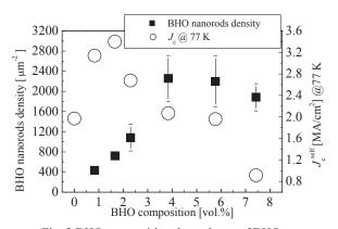
Fig. 2 BHO composition dependence of BHO nanorods density and  $J_{\rm c}^{\rm self}$  @ 77 K
