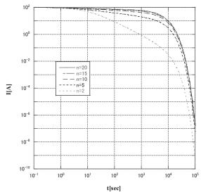
Fig.4 The property of the interrupting current
