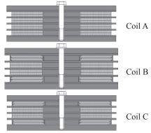
Fig.2 Schematic illustration of cross sections of test HTS coils
