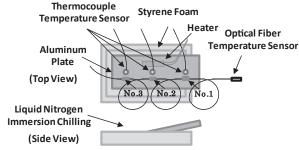
Fig.1 Schematic Illustration of Experimental Equipment
