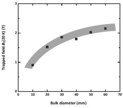
**Fig. 1.** Bulk diameter dependence of trapped field at 20 K at the center of bulk surface for the MgB<sub>2</sub> bulk samples with 10, 20, 30, 40, 50 and 60 mm in diameter and 10 mm in thickness.
