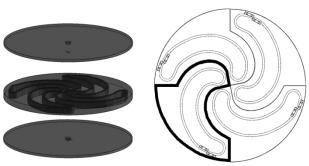
Fig.2 Contracture of Spiral Sector Coil
