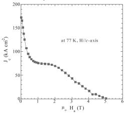
Fig.3 Field dependence of the critical current density ( $J_c$ ) of the Y-123 sample IG-processed in air, measured at T=77 K with H//c-axis. Note that record critical current density of 175 kA/cm<sup>2</sup> at self field and 77 K was achieved for the first time in Y-123 system.
