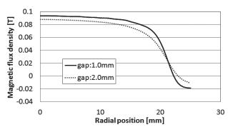
Fig.3 Influence of the gap length on magnetic flux density distribution
