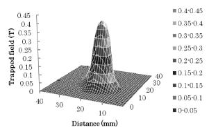
Fig.1 Trapped flux distribution of 30 mm diameter Y-123 bulk at liquid nitrogen temperature. Note that the maximum the trapped field value reached 0.41 T at 1.2 mm above the sample surface and around 0.45 T when it is measured directly on the bulk surface
