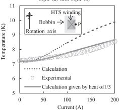
Fig.2 Comparison between experimental and calculation results on temperature variation at the position of P
