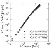
Fig.3 Measurement results of AC loss in test coils
