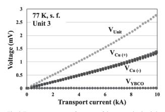
Fig. 2 Transport current performance of the current lead unit 3 (@77 K, s. f.).
