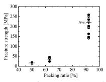
Fig.1 Fracture strength at room temperature of  ${\rm MgB_2}$  bulk samples with different packing ratios.
