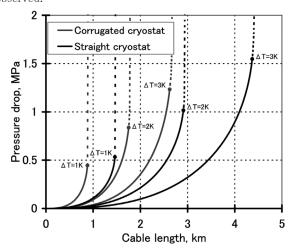
Behavior of  $\Delta p$  as a function of cryostat length in case of  $\Delta T$  = const, namely 1, 2, and 3 K. Straight cryostat I.D. is 60 mm, corrugated one is 60/66 mm. Cable O.D. is 40 mm in both cases. Heat leakage through thermal insulation is 1.2 W/m.
