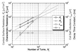
Fig. 2 Characteristic resistance ( $R_c$ ), contact surface resistance ( $R_{ct}$ ), decay time constant ( $\tau$ ), and coil self inductance ( $L_{coil}$ ) as a function of number of turns
