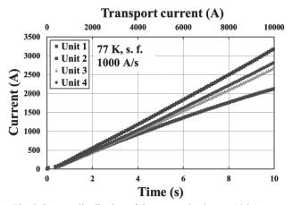
Fig. 3 Current distribution of the current lead up to 10~kA at sweep rate of 1,000 A/s.
