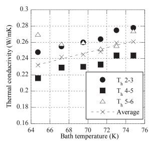
Fig. 2. Measured thermal conductivity of subcooled liquid nitrogen impregnated PPLPs.
