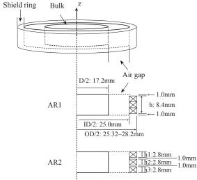
Fig.2 Arrangement of HTS shielding ring.
