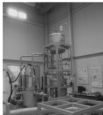
Fig.1 Cryocooler and pump system of CASER-2.
