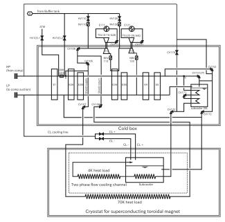
Fig.1 Schematic flow diagram of TREK experiment.
