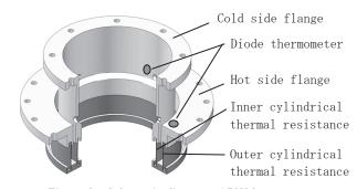
Figure 2 Schematic diagram of 70K heat meter
