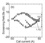
Fig. 1 Hysteresis loop of the screening field (Experimental results). (a) Coil-A. (b) Coil-B.
