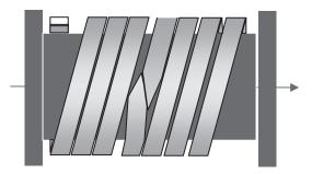
Fig.2 2-strand parallel conductor wound into a 1-layer solenoidal coil
