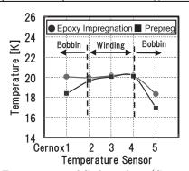
Fig.2 Temperature of Coil windings(Current 200A)
