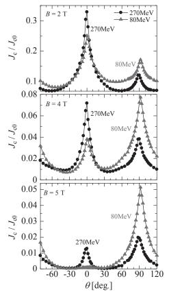
Fig1. Angular dependences of  $J_c$  at 84K for B = 2T, 4T, 5T
