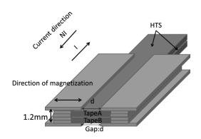
Fig.1 Arrangement of the HTS tapes
