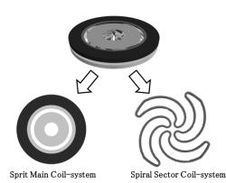
Fig.1 Schematic drawing of the Conceptual design of HTS cyclotron
