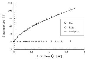
Figure 3 Cakibration test results of 70K heat meter
