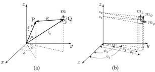
Fig. 1. (a) Magnetic moment m at point Q generates magnetic flux  $\Phi$  at point P (b) Dimensions of a ferromagnetic piece.
