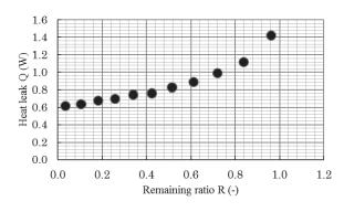
Fig. 2 Characteristics of heat leak Q and  $LN_2$  remaining amount ratio R of the bottle A
