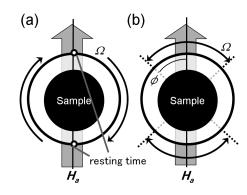
Fig.1 Two different types of modulated rotating magnetic fields. (a) unidirectional rotation type, (b) oscillation type.
