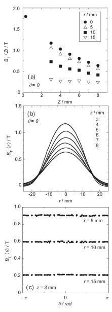
**Fig.1** (a) Height directional, (b) radial directional and (c) circumferential directional distributions of trapped magnetic field of MgB<sub>2</sub> bulk disk magnet at 20 K.
