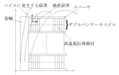
Fig.1 Schematic illustration of magnetic flux distribution in HTS coil
