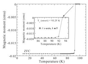
Fig.2 Superconducting transitions for specimens cut from various locations of single-domain Y-123 superconductor prepared in air with IG process.
