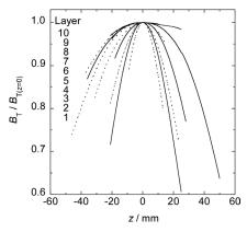
**Fig.2.** Standardized trapped field of multi layer bulk superconductor annuli
