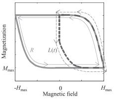
Fig. 1 Differences between magnetization losses given by eqn. (2) and eqn. (3)
