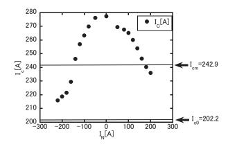
Fig.3 Critical currents of HTS tapes
