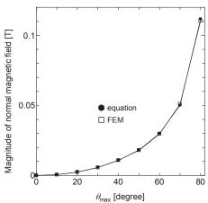
Fig. 2 Magnitude of normal magnetic field in each  $\theta_{\text{max}}$ .
