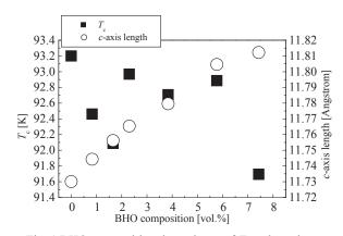
Fig. 1 BHO composition dependence of  $T_c$  and c-axis length for SmBCO films on LSAT
