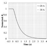
Fig. 1 Experimental results of normalized Bz vs. time functions from sudden discharge tests NI60
