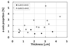
Fig.3 Thickness dependence of a-axis proportion
