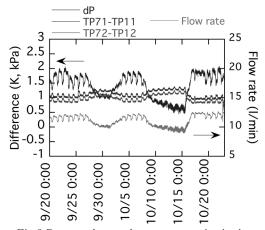
Fig.2 Pressure loss and temperature rise in the circulation test of the 5<sup>th</sup> cooling test.
