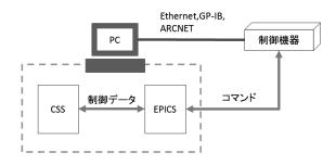
Fig.1 Schematic view of the magnetic field measurement control system.
