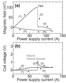
Fig.2 Experimental results for the paraffin impregnated uninsulated pancake coil. (a) Axial magnetic field at the coil center vs. power supply current. (b) Coil terminal voltage vs. power supply current.
