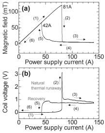
Fig.1 Experimental results for the dry wound uninsulated pancake coil.(a) Axial magnetic field at the coil center vs. power supply current. (b) Coil terminal voltage vs. power supply current.
