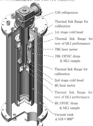
Figure 1 Test apparatus utilizing GM refrigerator to measure the thermal insulation performance of MLI
