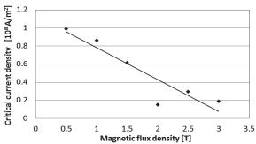
Fig. 2 Estimated  $J_C$ -B characteristics
