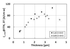
Fig.1 Thickness dependence of  $I_{c, min}$  at 77 K, 3 T
