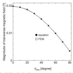
Fig. 3 Magnitude of transverse magnetic field in each  $\theta_{\rm max}.$
