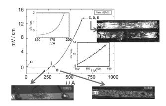
**Fig.1.** The state of tapes at over-current turning
