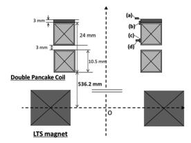
Fig.1 Schematic drawing of experimental setup and arrangement of Hall probes
