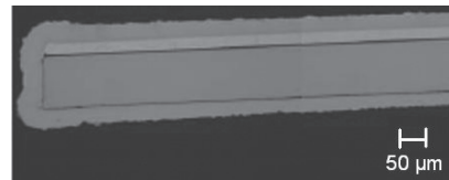
Fig. 1 Cross section of YBCO tape after Cu plating
