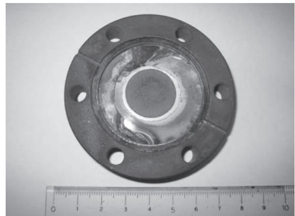
Fig.2 Photograph of an as-sintered MgB<sub>2</sub> bulk in the stainless steel flange.
