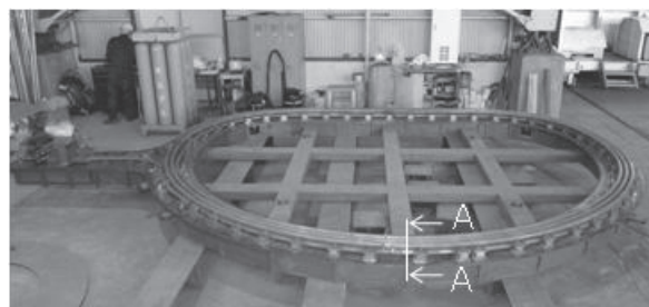
Fig. 3 Heat treated 1/3 scale winding.
