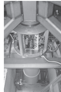
Fig.1. ISSP high speed rotational cryostat to study \Omega_{c1} [6].
