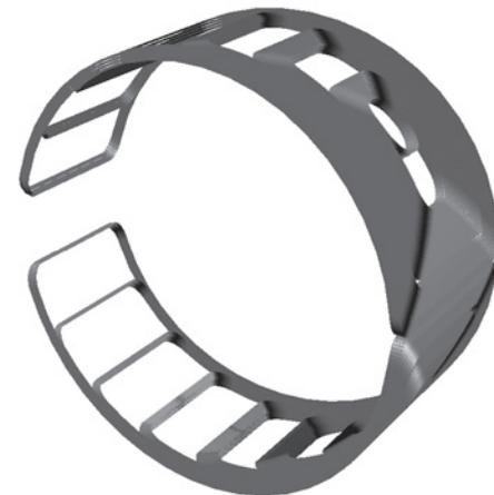
Fig. 2 Shape of designed magnet.
