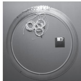
Fig.1 Photograph of φ 730 mm-class pancake coil
