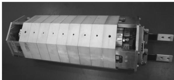
Fig.1. Photo of ILC quadrupole model.
