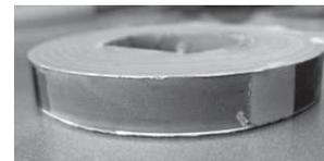
Fig.1 Single-pancake coil wound with an YBCO wide tape
