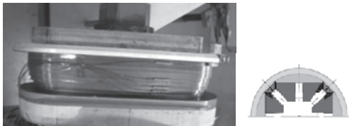
Fig.1 Y-model coil for motor application (left). Assumed half cross-section in the 4-pole 500kW Y-motor (right).
