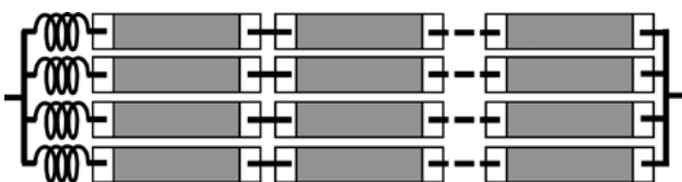
Fig. 2 Circuit diagram for the parallel connection of series-connected FCL elements, with using appropriate inductors.
