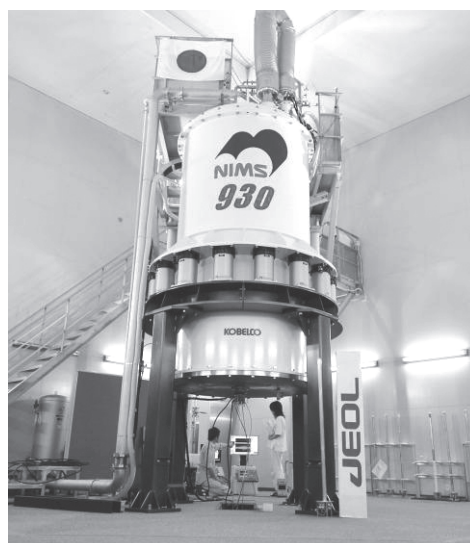
Fig. 1 930 MHz (21.8 T) NMR magnet in NIMS, Tsukuba.
