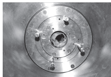
Fig.2 Bottom view of the OVC flange. The crushed RT bore can be seen in the center.
