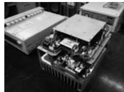
Fig. 4 100 A class current source by use of power MOS-FET (rippled current can be applied to the load).
