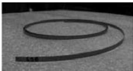
Fig. 1 Photograph of a YBCO tape (width: 3 mm).
