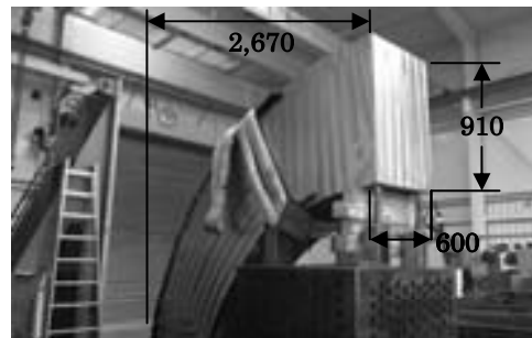
Fig.2 Manufacturing of Coil Case (Side Plate)
