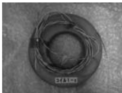
Fig.2 GdBCO-coil with epoxy impregnation. (inner diameter: 80mm, outer diameter: 153mm, height: 6mm)
