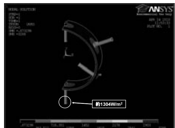
Fig.3 Heat flux distribution of supporting structure in simulation.
