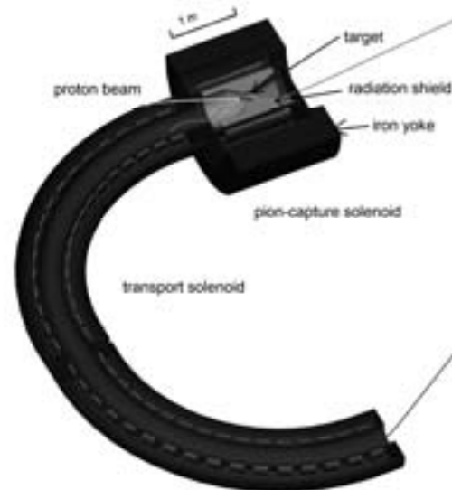
FIGURE 1. Schematic layout of the MUSIC solenoid magnets. Superconducting coils are indicated in red. Yellow line indicates proton beam injected onto the graphite target. Red trajectory indicates pions. Blue indicates muons from pion decay. Iron yoke and stainless steel radiation shielding are shown in brown and gray, respectively.
