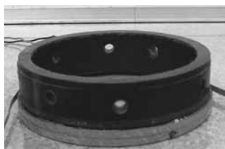
Fig. 1 Photograph of YBCO double-pancake coil.
