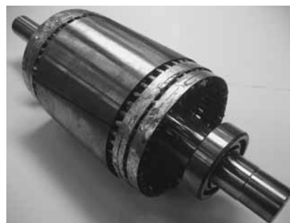
Fig. 2 Photograph of the HTS rotor fabricated with Bi-2223/Ag tape conductors [7].
