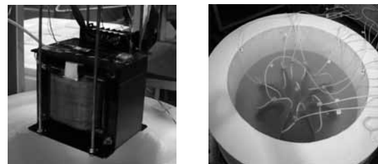
Fig. 2 DC model reactors composed of conventional copper coil and YBCO toroidal coil (8 double pancake coils).
