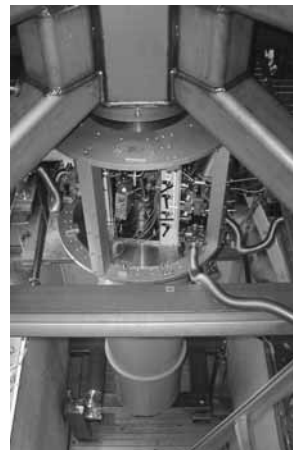
Fig.1 ISSP fast rotating cryostat lower frame with Dewar: view from upper space.
