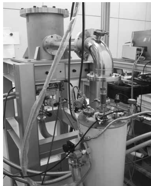
Fig.2 HCS with 1/2 inch insert tube for general superconductive apparatuses.
