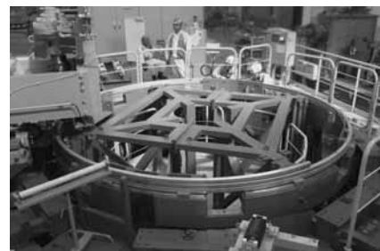
Fig. 2 Spooled 28-m long jacket for CS conductor
