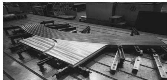
Fig. 1 Regular Radial Plate Segment.
