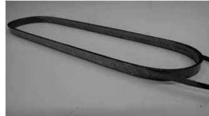
Fig. 1. Photograph of racetrack double-pancake coil made of YBCO coated conductor, which is insulated with polyimide tape.
